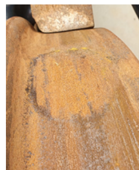
Figure 1 Scratches and small damages along the running surface (a), Flat spots formed by blocking the wheelset by seizure of the axle box, insufficient wagon braking or brake system jamming (b)
