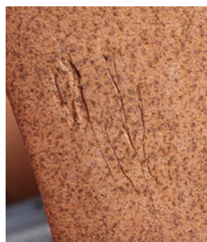
Figure 1 Scratches and small damages along the running surface (a), Flat spots formed by blocking the wheelset by seizure of the axle box, insufficient wagon braking or brake system jamming (b)
